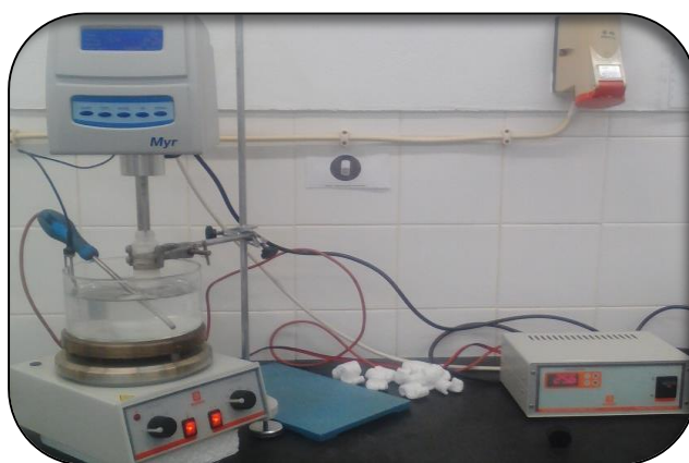
Figure 10: Viscosity measurement with the viscometer.
