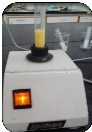
Figure 8: Vibration test with the vortex equipment.
