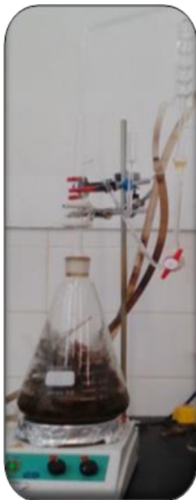
Figure 7: Extraction of EO by Clevenger apparatus.
